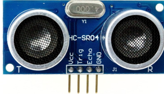
Figure otto.1 : The HC-SR04 sensor is an ultrasonic model composed by a speaker and a microphone. It can be used to measure distances.
