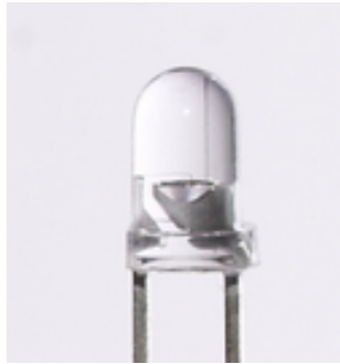
Figure sette.1 To tell which lead of the LED is the cathode look through its body: the thickest lead is the cathode (on the right in this picture). The picture has been taken from Wikipedia .
