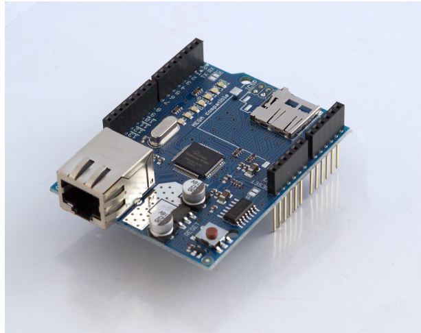
Figure sei.1 The Arduino Ethernet shield is a board that plugs on top of an Arduino board. This shield has an RJ45 connector to connect it to a plug via an RJ45 cord and a SD card slot. There exists shields with WiFi capabilities.
